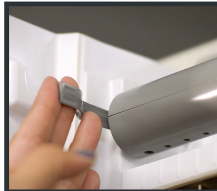
Remove the distribution tube, depressing both side tabs.
