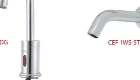
The CEF-1D series sensor faucets are single-hole, dual temperature, deck-mounted and come with vandal-resistant 8.3 L/min (2.2 GPM) aerators (unless otherwise stated), AC/DC transformers, control modules, mechanical mixing valves, G  $\frac{1}{2}$ " flexible supply hoses and G  $\frac{3}{8}$ " adapters. They can also run on batteries as a standalone solution.
