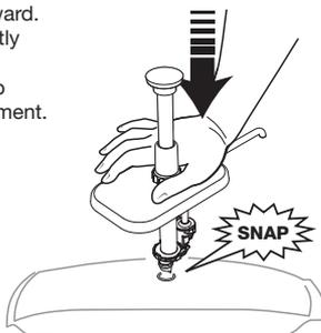
*Pump is fully engaged when top surface of pouch fitment touches pump connector rim.*
